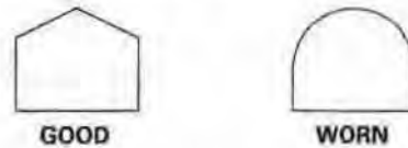
Example of synchro ring teeth
