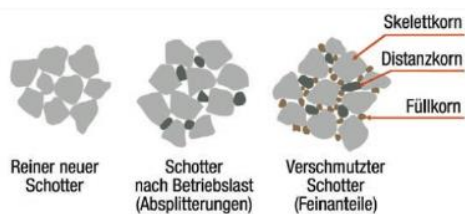
Figure 8. Formation of fine material in between larger particles. (Angerhn, 2015)
